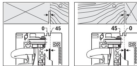
The 0° cut mark (9) indicates the position of the saw blade when making a right-angled cut. The 45° cut mark (8) indicates the position of the saw blade when making a 45° cut. For a precise cut, place the circular saw against the workpiece as shown in the figure. We recommend making a test cut.
