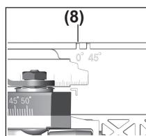
Use only cut marks (8) when making a right-angled cut and a 45° cut with the guide rail.
