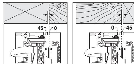
The 0° cut mark (8) indicates the position of the saw blade when making a right-angled cut. The 45° cut mark (9) indicates the position of the saw blade when making a 45° cut. For a precise cut, place the circular saw against the workpiece as shown in the figure. We recommend making a test cut.
