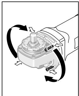
The machine head can be rotated with respect to the machine housing in 90° steps. In this manner, the On/Off switch can be brought into a more convenient position for special working situations, e. g., for cutting operations using the cutting guide with dust extraction protection guard 20 or for left-handed persons.
