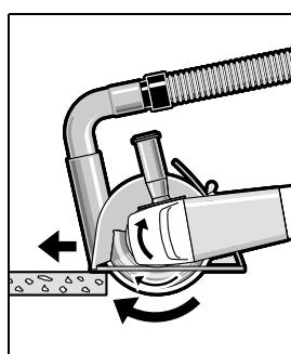
Switch on the machine and place the front part of the cutting guide on the workpiece. Slide the machine with moderate feed, adapted to the material to be worked.
