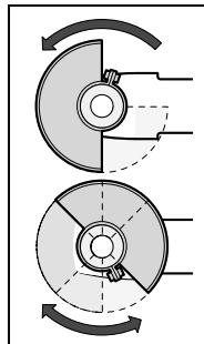
Place the protection guard **7** on the spindle collar. Adapt the position of the protection guard **7** to the requirements of the work step. Lock protection guard **7** by tightening locking screw **8** with combination spanner **4**.
